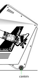
• When moving the main unit, lift the rear frame holding by the seat height lock knob, and roll the casters.
